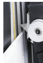
Universal turret cutting head with automatic blade disengagement at the end of cut
