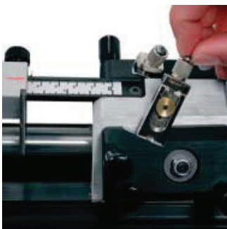
The blade holder is manufactured using high precision technology. It allows you to easily alter the blade depth by simply turning the adjustment screw to reduce or increase depth and ensures a perfectly straight cut at all times. Cuts mats of varying thickness from paper to mat boards up to 3.5mm (8 ply) thick.
